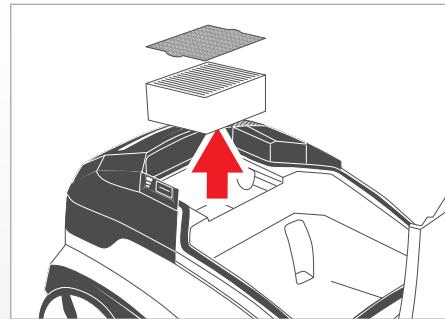
**ⓘ** When cleaning, do not use any brushes or implements which could damage the filter ribs. Before inserting back into the appliance, the filters must be completely dry.
