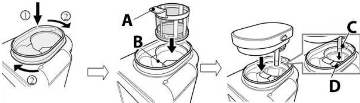
Place the grinding/brewing basket, until you hear a click sound (1) turn it clockwise until the container latches.
