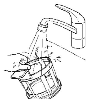
Clean the filter under running water and dry it after this.
