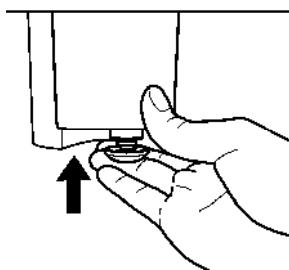
Press the drip stop and clean it with running water, then dry it.
