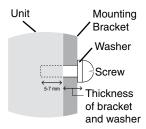
NOTE: Tighten all screws. (recommended Fasten Force: 98 - 137N•cm)
