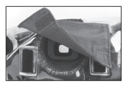
When the camera is not in use, fold the eyepiece flap over the eyepiece to protect the eyepiece from the elements
