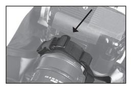
Step 4: IMPORTANT - The Lens Strap supports the camera's weight when the Hydrophobia Camera Strap is used. If the Lens Strap is not properly clipped around the lens, neither the camera nor the lens will be secured inside the rain cover. Carefully turn the camera over. Wrap the Lens Strap snugly around the lens, close to the camera. Ensure that the buckle and strap are positively connected around the lens.
