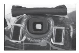
**Step 6:** Insert the Hydrophobia eyepiece (attached at Step 1) through the neoprene eyepiece port on the back of the Hydrophobia. This keeps a weather-resistant seal around the eyepiece and an unobstructed view through the camera.
